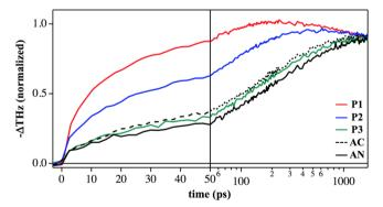
Figure 2. OPTP traces of P1 (red), P2 (blue), P3 (green), AC (dashed black), and AN (solid black) are normalized based on their best fit amplitudes from eq 2 to compare the overall ultrafast dynamics as a function of linker length. In each case, the porphyrin was photoexcited with 400 nm light at a fluence of  $100 \ \mu J/cm^2$ .
