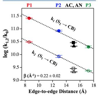
**Figure 3.** Plot of the common log of the extracted rate constants  $k_1$  and  $k_2$  versus edge-to-edge distance. Their associated standard deviations are displayed as well. The best fit lines for **P1**, **P2**, and **P3** are shown with dotted black lines.
