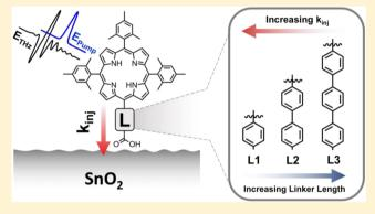
linker. We find a clear correlation between linker length and injection rates, providing insights that will be exploited in the optimization of dye-sensitized photoelectrochemical cells.
