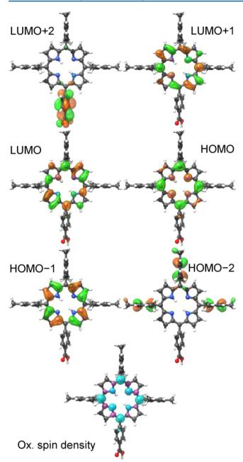
**Figure 4.** DFT frontier orbitals of **P1** (top) and the spin density of the singly oxidized state (bottom), where cyan and magenta represent spin up and down, respectively. Analogous isodensity plots for the other dyes are found in Figure S5.
