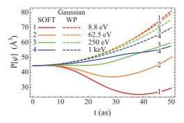
FIG. 7. (Color online) Participation function evaluated with the SOFT (solid curves) and Gaussian WP (dashed curves) density for four different values of the initial translational kinetic energy: 8.8 eV (1, red curve), 62.5 eV (2, orange curve), 250 eV (3, green curve), and 1000 eV (4, blue curve).
