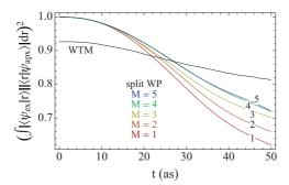
FIG. 9. (Color online) Overlap of the spatial densities between those from the SOFT method and WTM and the SOFT and split WP methods as a function of time. The initial overlap of the WTM and the SOFT method is not unity due to noise in sampling the initial state.
