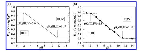
*Figure 5.* Pourbaix diagram for complex 1 in aqueous solutions, obtained (a) from free energy calculations of redox potentials at the DFT B3LYP/cc-pVTZ(-f) level of theory and (b) from experimental data (the circles) from ref 18.
