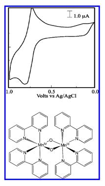
*Figure 1.* Cyclic voltammogram (top) for a 1 mM solution of complex **1** (bottom) in phosphate buffer at pH 3.78 as reported in ref 18.
